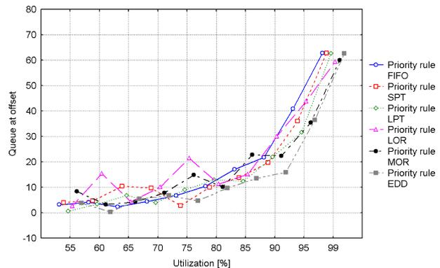
Fig. 4. Queue at offset versus resource utilization.
